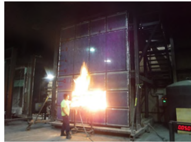
Photo No. 13 Ignition of Window Burner
