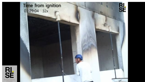
Test 1 - Exposed timber: 53.8 m 2
