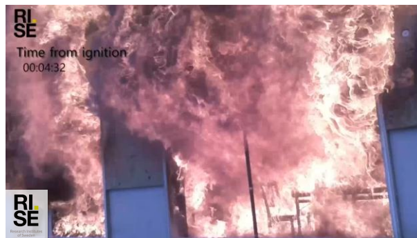
Test 5 - Exposed timber: 97.2 m 2
