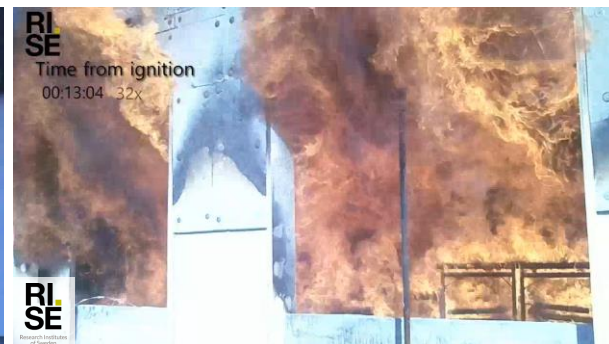
Test 3 - Exposed timber: 96.2 m 2
