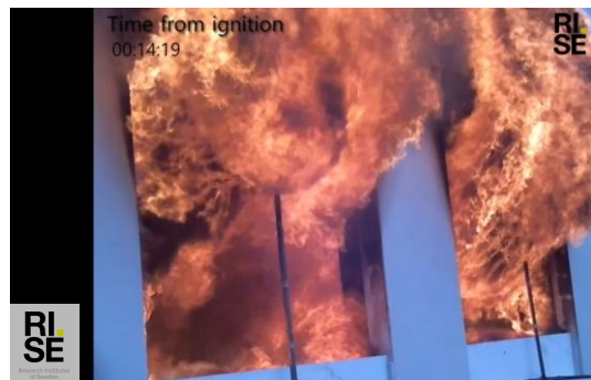
Test 1 - Exposed timber: 53.8 m 2
