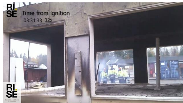
Test 4 - Exposed timber: 77.9 m 2
