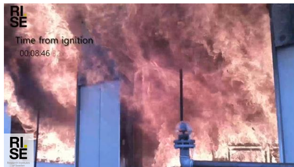
Test 2 - Exposed timber: 91.2 m 2
